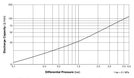
1. Differential pressure is the difference between the inlet and outlet pressure of the air vent. 2. Capacities are equivalent capacities of air at 20 °C under atmospheric pressure.
